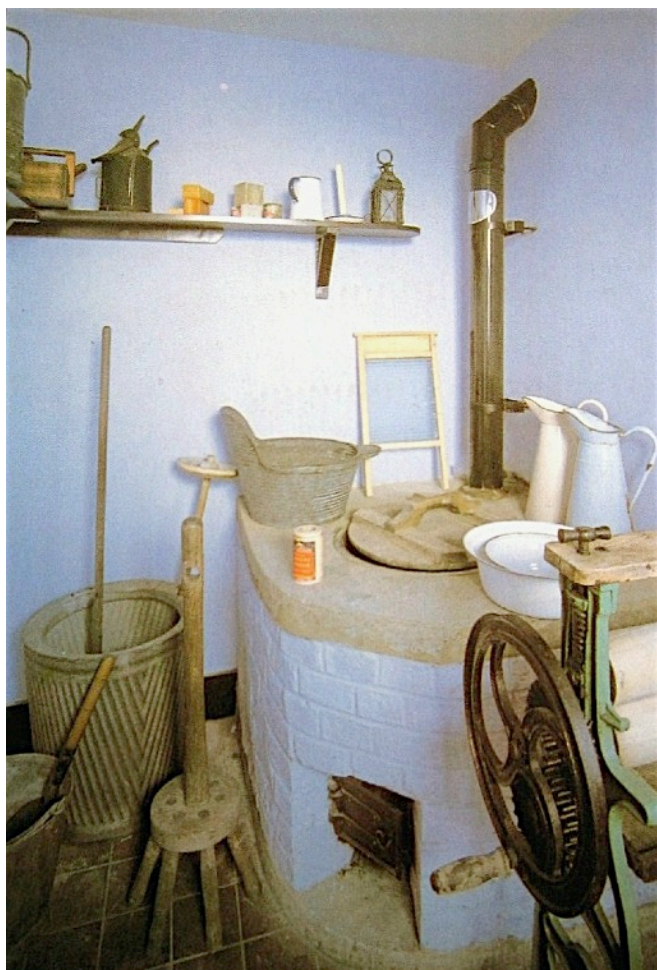
A late nineteenth century laundry with a tub and its dolly, a brick built copper and mangle.
